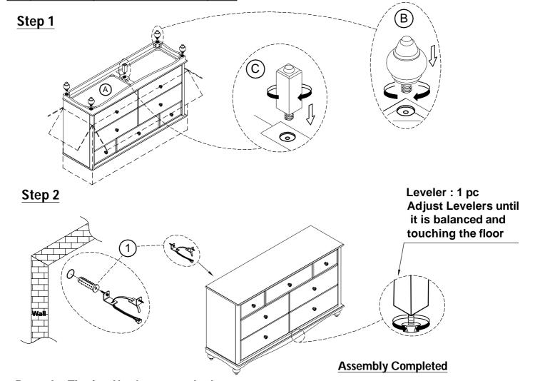
Remark: Tipping Hardware attached to the back stretcher
